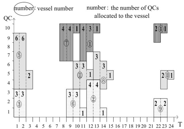
**Fig. 7** Single objective 2 (minimizing the number of moves by all of the QCs)—allocation of QCs
