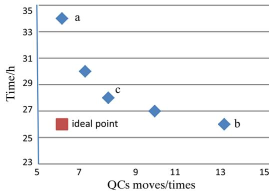
**Fig. 8** Pareto-optimal solution. Time: total time for which all vessels are in port, QC move: Number of QC moves
