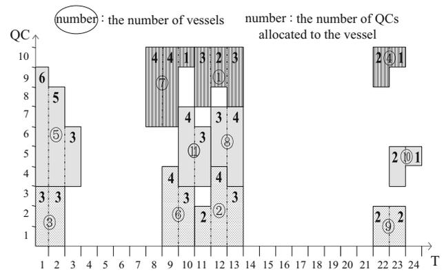
**Fig. 9** Multi-objectives (minimizing the total time spent by all vessels in the port and minimizing the number of moves made by all QCs)—allocation of QCs
