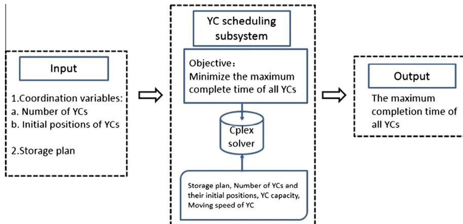
Fig. 3. Model of YC scheduling subsystem.
