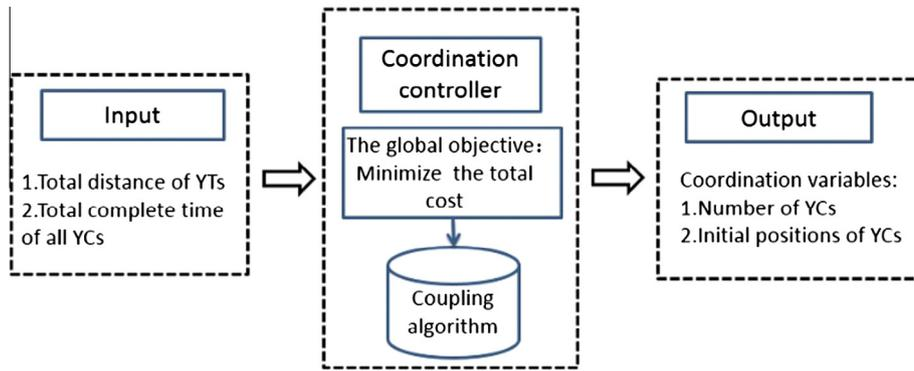
Fig. 4. Model of coordination controller.
