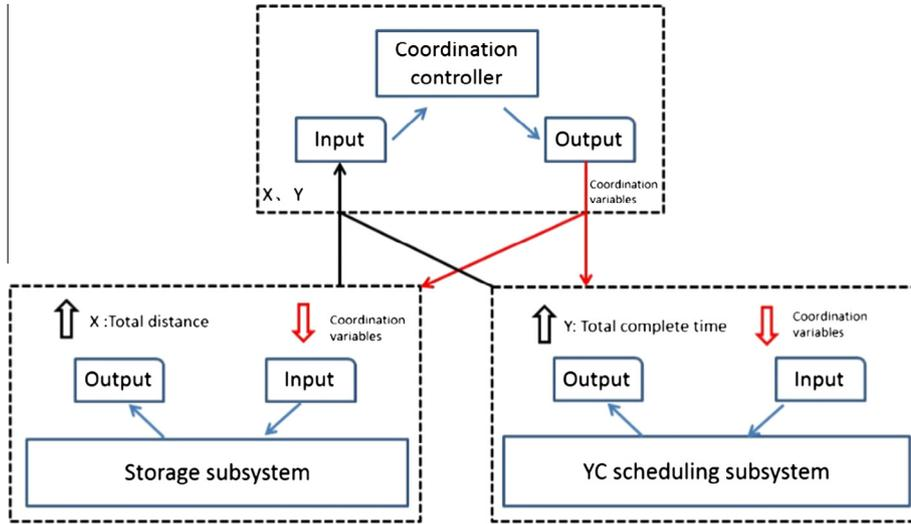
Fig. 1. Framework of coordinated model of yard.
