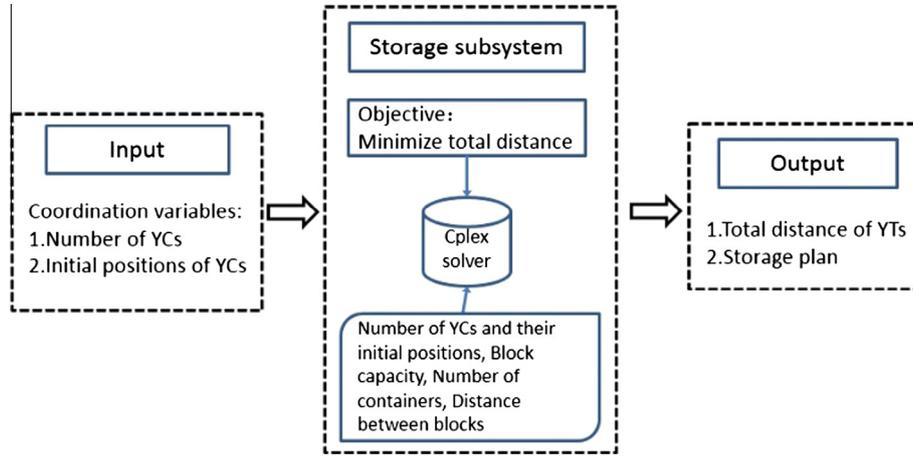
Fig. 2. Model of storage subsystem.
