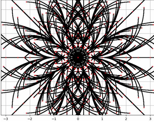
Figure 2: The example of the motion primitives. The red dots are the states; the black lines/curves are trajectories between states.
